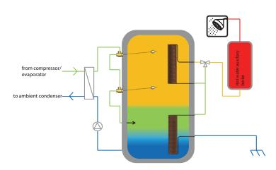
The valve is installed directly on a storage tank inlet, where it switches the flow direction of the incoming flow based on the temperature difference between the incoming flow and the temperature inside the tank, directing it either into the tank or through its bypass outlet to a different position in the storage tank.
